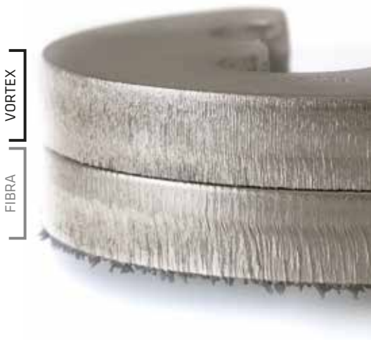
3/8" stainless steel cutting comparison between 4kW fiber laser with and without Vortex feature
