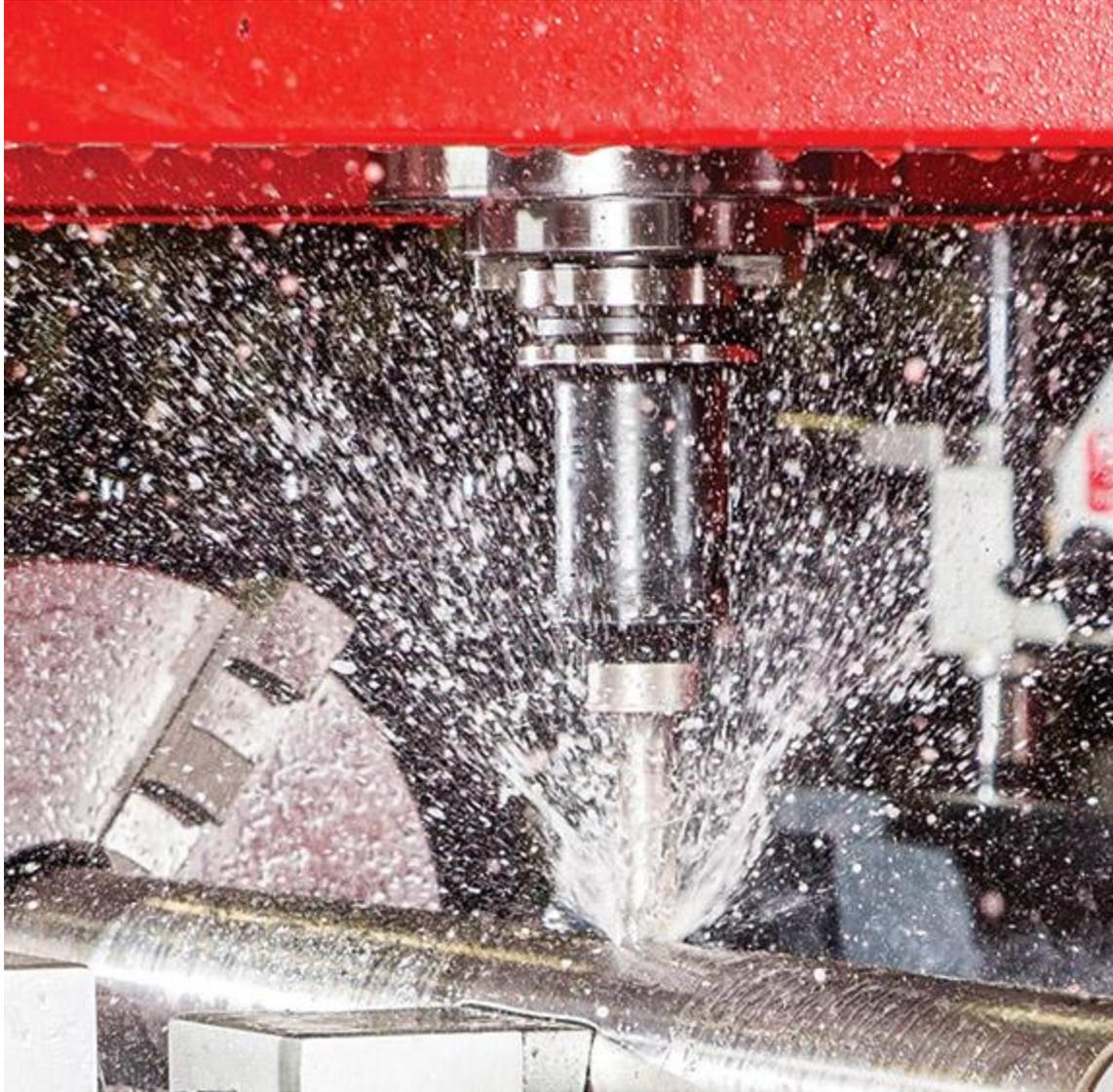
*Coolant helps the spindle achieve heavier cuts, while cutting at higher feed rates, and perform deep drilling with better surface finishes.*
